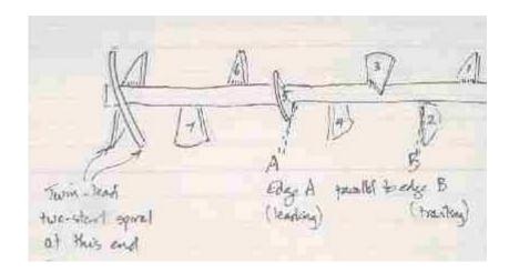
This photo shows one of the long-ago sketches made when building the first pugmill. Blades 1 to 7 resemble a continuous single spiral of pitch approx 150 mm, with alternate sections removed. One revolution of the spiral occupies about 150 mm.
