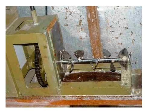
In this picture you can see the auger assembled in the main chassis. Notice the thrust bearing at the left end of the auger shaft, and the 50tooth sprocket which drives the shaft. This big sprocket is mounted on a steel bush with a wide flange, specially made for the job. The bush is held onto the shaft by a 6 mm drive-in "Sellock" pin through a hole in the shaft
