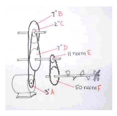
The speed reduction in this model was done using vee belts and pulleys, then a chain and sprocket drive to the auger. Pulley A on the motor (3 inch) drives pulley B (7 inch) on a layshaft. Then C drives D, on a second layshaft which also carries a toothed sprocket E (11 teeth)
