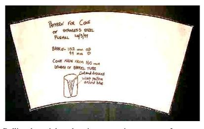
If not, you can make it yourself. In my case, a paper template of the necessary shape was made up, then a 160 mm length of the larger pipe was slit along one edge and opened out a little. With the paper template wrapped around the pipe, the pipe was marked then cut away where necessary.
