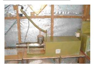
This picture shows one version of a home-made pugmill, at present used for terracotta clay. The barrel is made from stainless pipe as you can see. The feed hopper on this model was made from the same circular pipe as the barrel, an idea that seemed right at the time. But in a later version, you'll notice the hopper is nearly square. Square is better. Easier to feed in big chunks of clay cut from a fresh block.
