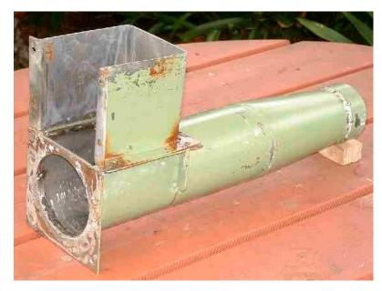
The hopper is a simple folded box made up from lighter gauge stainless sheet., fixed to the main barrel with six small bolts. The rusty stains are from these bolts, sold as "stainless" but they corroded anyway.
