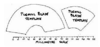
Stainless steel plate 3 mm thick is about right. The blades can be made a millimetre or two oversize if it helps, and trimmed back to size with an angle grinder later.
