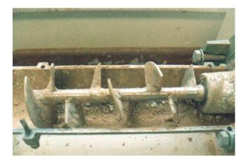
You'll notice the blades arranged in a spiral pattern along the shaft. The spiral in this case has a right-hand twist. Seen from the exit end, the shaft would have to rotate clockwise. If you are designing your own machine, this is something to keep in mind. Left-handed spiral or right-handed? It depends on the motor and drive you select.
