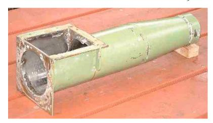
Here is the barrel assembly, ready to bolt onto the main chassis. Note the four bolt holes near the corners of the square plate, and the smaller holes around the top flange to fix the hopper in place.
