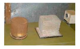
To close off the hopper and keep it damp when not in use, try a block of soft foam plastic trimmed to shape, and glued to a thin wooden cap. Just wet the plastic, squeeze it out, and insert the block in the hopper with the wood on top as a lid. Rest the plunger on the lid to keep it all in place. This photo shows two of these, one for the pugmill with the circular hopper, and the other for the rectangular one.
